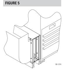
**NOTE FOR UPFLOW INSTALLATIONS:** Provide support under the outer housing to ensure the quality of the seals (see **Figure 5**).
