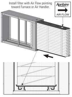
Align filter in top and bottom rails and slide into place. Reinstall door.
