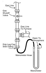
Measuring Inlet Gas Pressure (Alt. Method)
