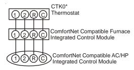
System Wiring using Four-Wires
