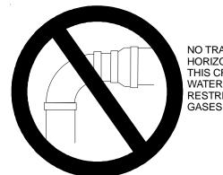
NO TRANSITION ON HORIZONTAL PLANE, THIS CREATES A WATER TRAP AND RESTRICTS FLUE
