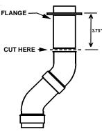
**Vent/Flue Pipe Cuts**
