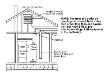
Figure A.9.3.3.1(1)(b) All Combustion Air From Outdoors through Ventilated Attic.
