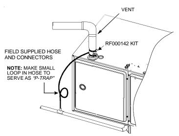
**NOTE:** When using the horizontal alternate vent configuration, you must use the RF000142 vent drain kit.
