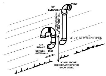
Combustion Air Intake may also be snorkeled to obtain 12" min ground clearance.
