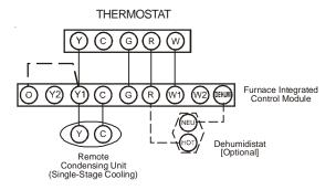
Thermostat - Single-Stage Heating with Single-Stage Cooling
