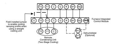
Thermostat - Two-Stage Heating with Two-Stage Cooling
