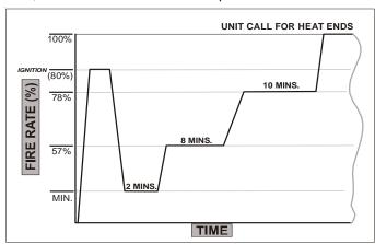
Operation with Conventional 1-Stage Thermostat (DIP switch selects 1-Stage heat)
