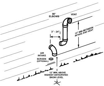
Alternate Horizontal Vent Termination (Dual Pipe)
