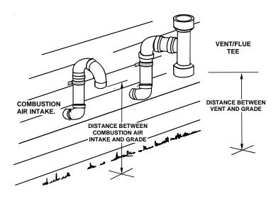
For all side wall horizontally vented gas fueled equipment installed in every dwelling, building or structure used in whole or in part for residential purposes, including those owned or operated by the Commonwealth and where the side wall exhaust vent termination is less than seven (7) feet above finished grade in the area of the venting, including but not limited to decks and porches, the following requirements shall be satisfied:
