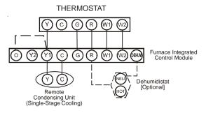
Thermostat - Two-Stage Heating with Single-Stage Cooling
