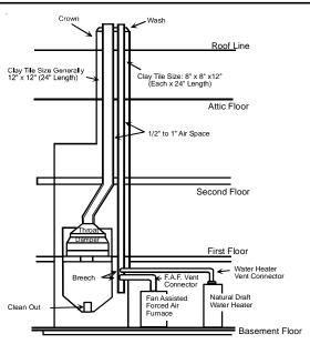
Typical Multiple Flue Clay Tile Chimney
