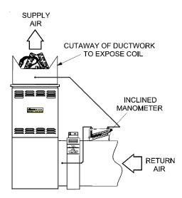
Checking Static Pressure (80% Furnace Shown, 90% Similar)
