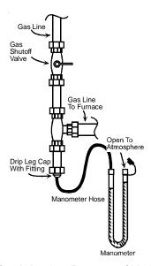
Measuring Inlet Gas Pressure (Alt. Method)
