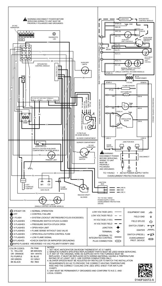
Wiring is subject to change. Always refer to the wiring diagram on the unit for the most up-to-date wiring.
