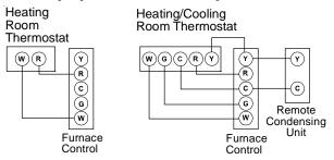
Typical Field Wiring (24 VAC Control Circuit)
