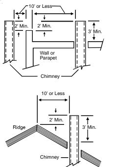
Termination 10 Feet Or Less From Ridge, Wall or Parapet
