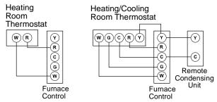
**Typical Field Wiring (24 VAC Control Circuit)**
