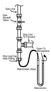
Measuring Inlet Gas Pressure (Alt. Method)
