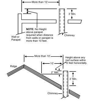
Termination More Than 10 Feet From Ridge, Wall or Parapet
