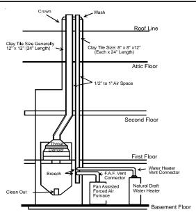
Typical Multiple Flue Clay Tile Chimney
