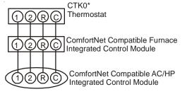
System Wiring using Four-Wires
