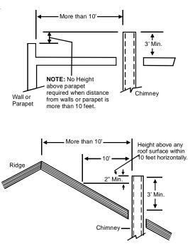
Termination More Than 10 Feet From Ridge, Wall or Parapet
