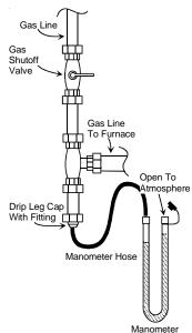
Measuring Inlet Gas Pressure (Alt. Method)
