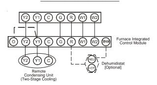
Thermostat - Two-Stage Heating with Two-Stage Cooling
