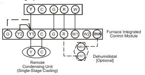
**NOTE:** To apply a single-stage Heating Thermostat, the thermostat selector switch on the Integrated Control Module *must* be set on single-stage.
