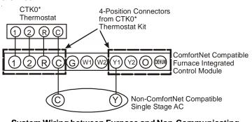
System Wiring between Furnace and Non-Communicating Compatible Single Stage Air Conditioner
