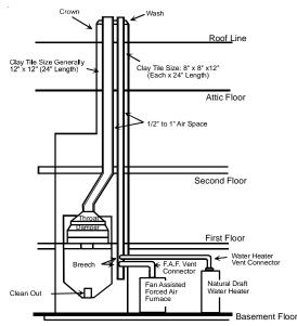
Typical Multiple Flue Clay Tile Chimney
