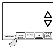
Upon entering the advanced menus, the Advanced Fault Menu is displayed. The display will change to the Fault Screen and indicate any faults that may be present in the indoor or outdoor equipment. If a fault is present, the Fault Screen will show the equipment and an error code with a description of the fault.
