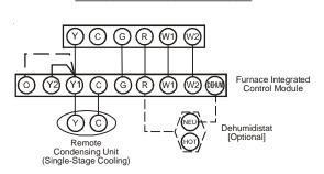
Thermostat - Two-Stage Heating with Single-Stage Cooling
