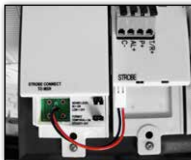
Strobe connection is clearly labeled for quick, simple installation.
