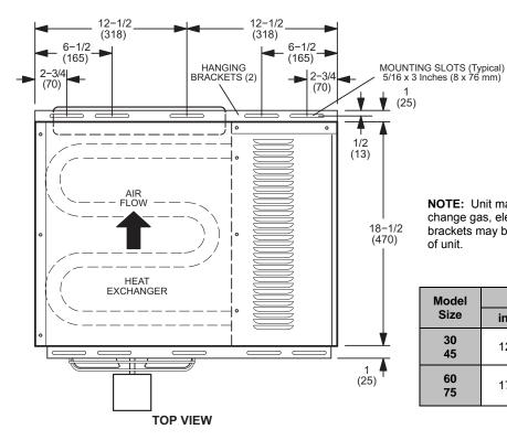
**NOTE:** Unit may be rotated 180° top for bottom to change gas, electrical and flue positions. Hanging brackets may be installed on either top or bottom of unit.
