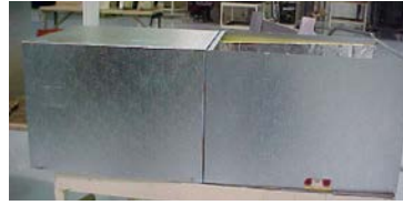
Front of blower (left) connected to a HD coil (right).
