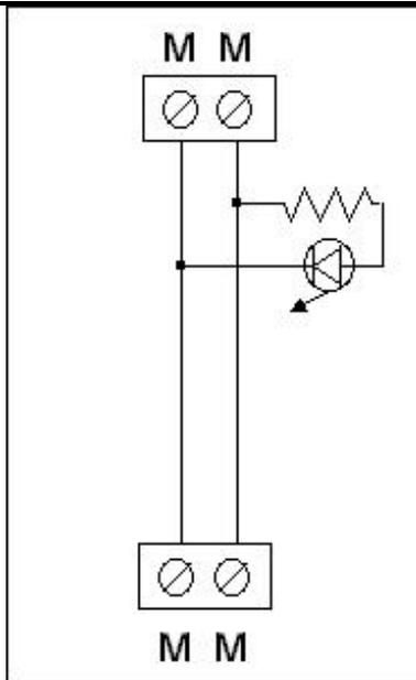
MM- 24vac input to damper motor
