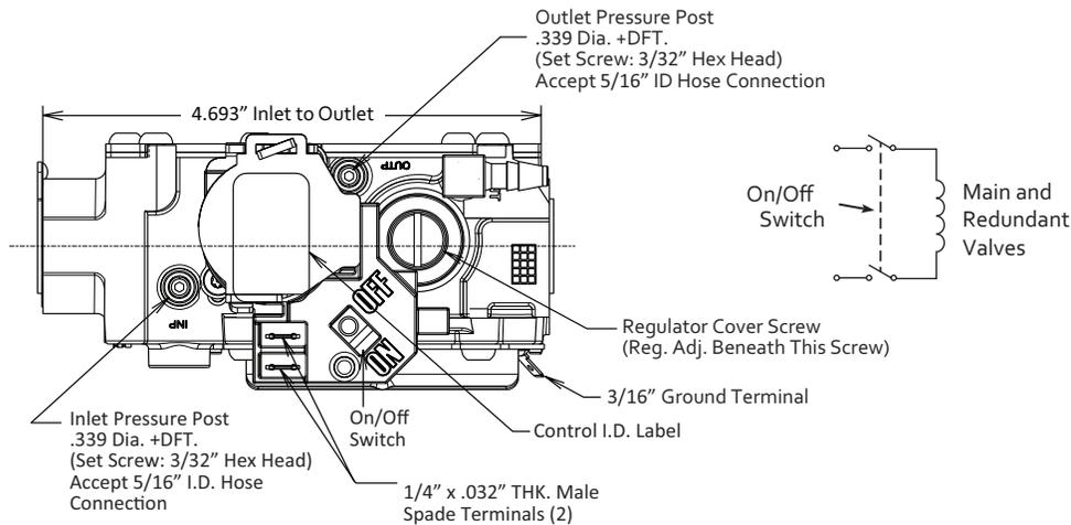
**Fig. 1 - Single Stage Valve Features, Terminals and Wiring**
