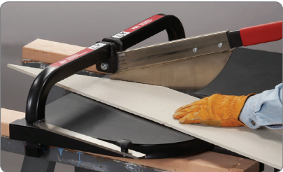
Scribe desired angle on fiber cement siding plank and feed it into the guillotine blade as you cut.
