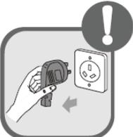
Turn off the unit or cut off the power supply before cleaning the unit, otherwise electric shock or injury may happen.
