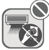
Never start up or shut off the air conditioner by means of directly plug or unplug the power cord.
