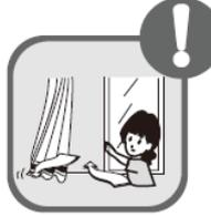
If refrigerant leakage happens during installation, please ventilate immediately. Poisonous gas will emerge if the refrigerant gas meets fire.
