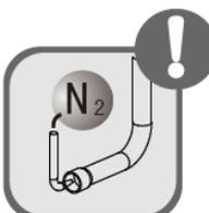
Never fail to comply with the nitrogen charge requirements. Charge nitrogen when welding pipes.
