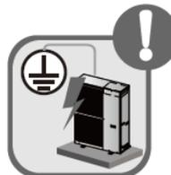
Make sure the unit can be earthed properly and soundly after plugging into the socket so as to avoid electric shock. Please do not connect the ground wire to gas pipe, water pipe, lightning rod or telephone line.
