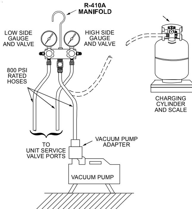
2. Start the vacuum pump and open the shut off valve to the high vacuum gauge manifold only. After the compound gauge (low side) has dropped to approximately 29 inches of vacuum, open the valve to the vacuum thermocouple gauge. See that the vacuum pump will blank-off to a maximum of 25 microns. A high vacuum pump can only produce a good vacuum if its oil is non-contaminated.
