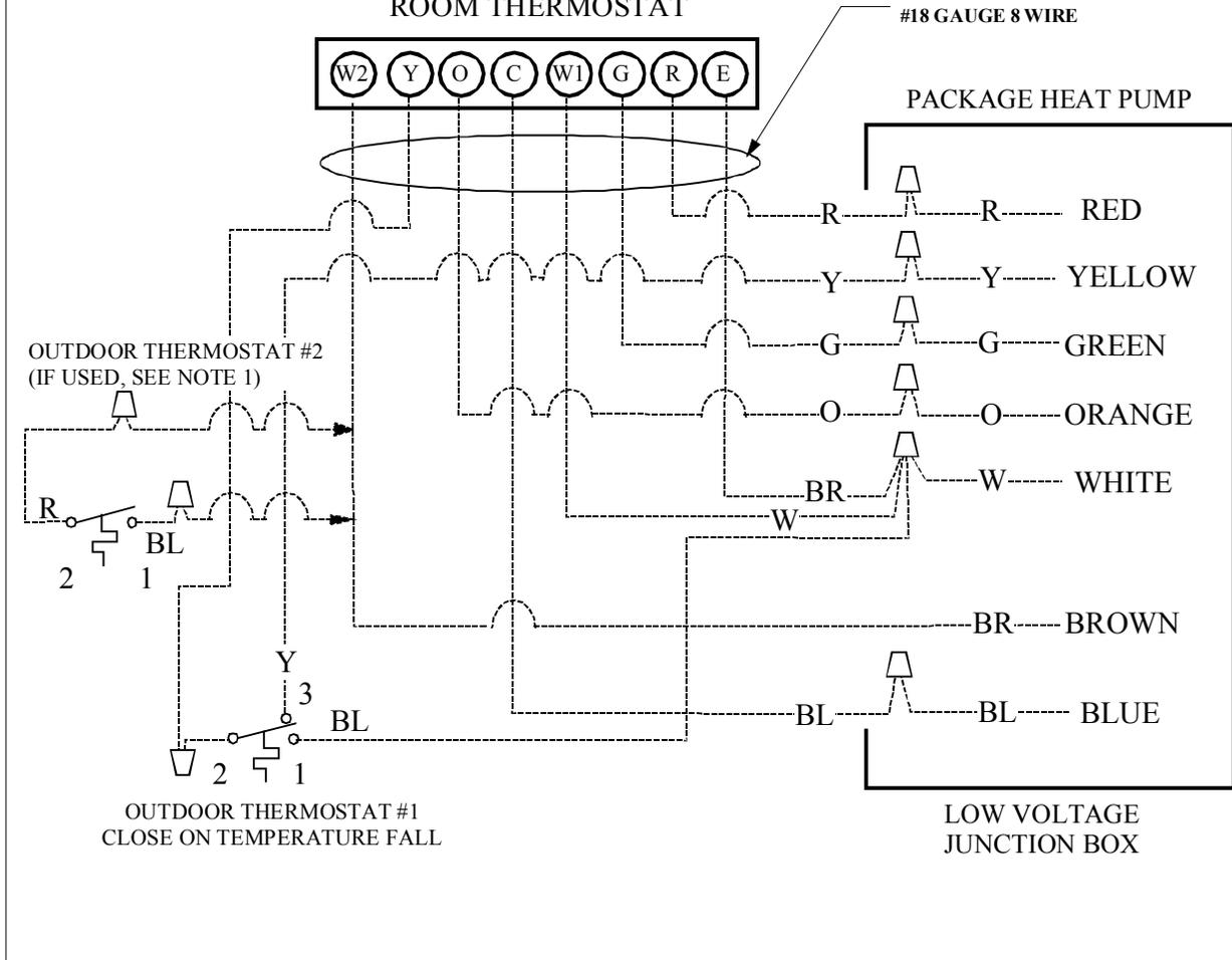
For outdoor temperatures below 0° F with 50% or higher relative humidity, set outdoor thermostat at 0° F
