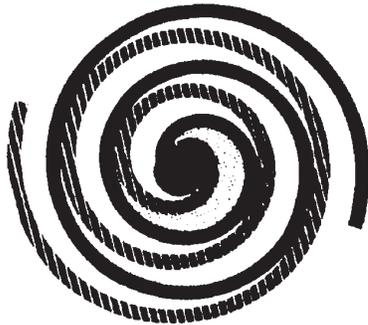
As this motion occurs, the pockets between the two forms are slowly pushed to the center of the two scrolls while simultaneously being reduced in volume. When the pocket reaches the center of the scroll form, the gas, which is now at a high pressure, is discharged out of a port located at the center.
