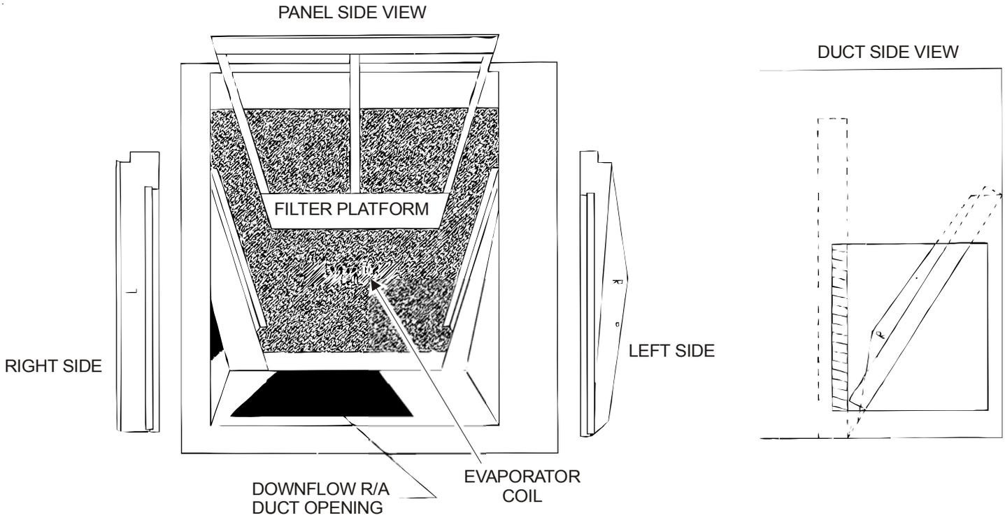
**Filter Size: 14" x 25" x 2" (Requires 2 filters) - Measurement in inches**
