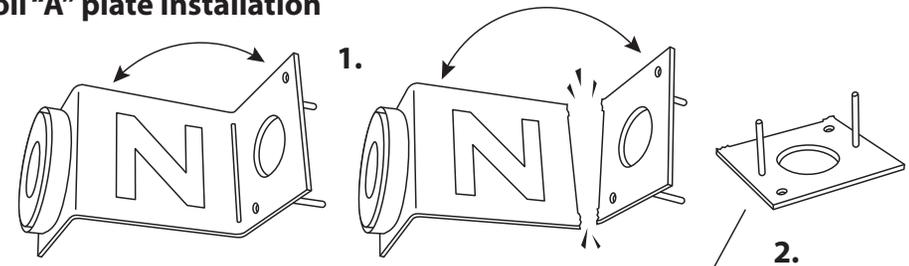
1. Snap the **"Z" bracket** apart by bending.
