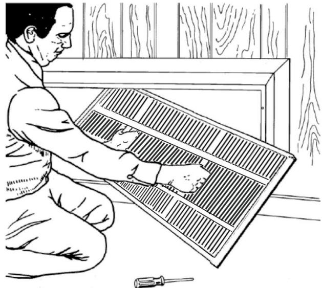
Fig. 2 - Aligning Grille with Wall Sleeve
