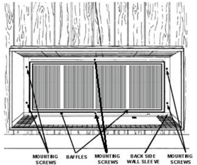
Fig. 4 - Securing Grille to Wall Sleeve
