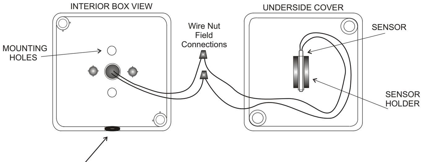
**NOTE: Orient the box housing with the Wire Entrance hole/Grommet facing down!**
