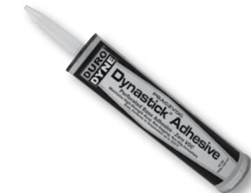
PBACZVOC contains Zero VOC and is ideal for use with PBH Dynastick Hangers. Place a small amount of PBACZVOC on a perforated base and firmly press the hanger against the duct surface. Allow the PBACZVOC mastic to dry, then, impale the insulation over the hanger nail and slip on a locking washer. Duro Dyne PBACZVOC adheres to concrete, metal or wood surfaces and performs in Temperatures Up To 225 °F.
