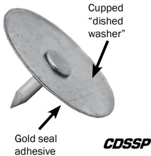
Capacitor Discharge Gold Seal (CDSSP) pins were designed to work perfectly with our Capacitor Discharge Spotwelders. They feature a heat activated gold adhesive on the underside of the washer which secures the pin to the liner facing during the welding process. CDSSP pins are manufactured from 12 gauge steel and feature a "dished washer". Do not store at or above 110°F or pins may stick together.
