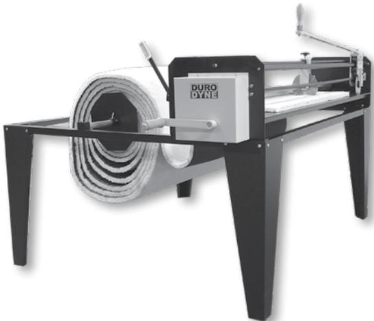
The LSU Advance Liner Sizer will help size and cut duct liner more efficiently than ever thought possible with a hand operated machine. It's enhanced features, make it possible to cut cotton fiber insulations, filter media, rubberized products and other unusual materials. The cross cut and slitter blades are mechanically gear driven to spin while cutting. This spinning action shears the material to create precise cuts in the most difficult of substances.
