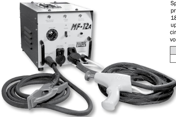
Special design welding transformers allow the MF12A to deliver more power, precisely timed to the welding tip. The MF12A will weld pins from 1/2"-2" on 18-28 gauge; weld performance for pins longer than 2" may vary dependent upon voltage, amperage and cable length. Proven solid-state weld control circuitry guarantees years of reliable, troublefree service in your shop. Input voltage: 208-230 V 60 HZ single phase. 60 amp service.
