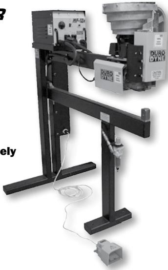
The FPP4 works in conjunction with the Duro Dyne MF12A compact pinspotter (sold separately). The FPP-4 is fully assembled for pneumatic and electronic controls to allow the MF12A welding source to be utilized as both a hand held pinspotter and a fixed head pinspotter. This provides the customer with greater capabilities at a lower cost. The MF-12A when used with the FPP4, will weld pins from 1/2 inch to 2 inches long on 18 to 28 gauge.
