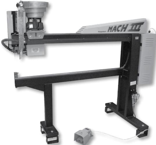
The FG Mach III Pinspotter was designed utilizing the best of current technologies to provide greater power and reliability for insulation fastening. The inherent minimal material handling and the use of welded pins will insure your shop a cost efficient, quality product. Our upgraded FG Mach III machine is capable of welding pins up to 4" to address the higher R-value insulation now being specified throughout the industry.
