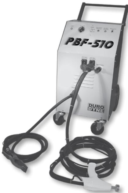
The PBF will weld pins from 1/2"-2" on 16-28 gauge; weld performance for pins longer than 2" may vary dependent upon voltage, amperage and cable length. It requires 220 volt, 50 to 60 hz service fused for 100 amps. Place a pin on the magnetic tip, insert the pin through the insulation, give the pin a 1/4 twist and depress the trigger switch. For PN type fasteners use a TP2 tip.
