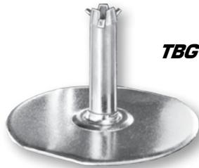
Tripod Bangers feature three prong jaws for added stability when fastening the banger to the sheet metal. They are 10 gauge and zinc chromate plated.
