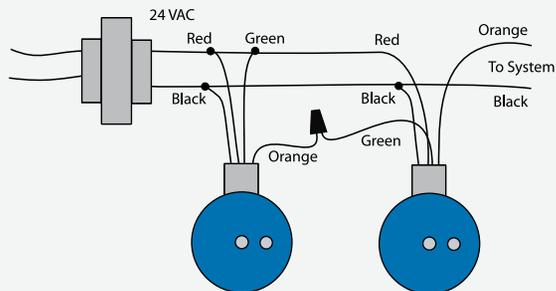
The contacts of the Wet Switch's relay may be wired to use multiple Wet Switches. The drawing above shows the contacts interrupting the 24 VAC signal when either Wet Switch® gets wet.
