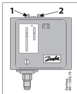
1. Set Cut In by adjusting range screw. Turn the screw clockwise to lower the set point.
