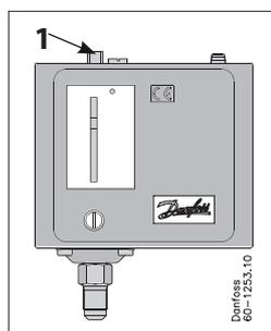
1. Set Cut Out by adjusting range screw. Turn the screw clockwise to lower the set point.
