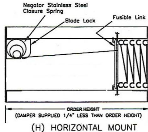
HORIZONTAL MOUNTING MODEL INCLUDES STAINLESS STEEL NEGATOR SPRINGS AND BLADE LOCKS
