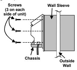
Figure 10 - Chassis Installation View 2
