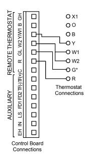
Figure 20 - Wiring Schematic for Straight Cool Unit
