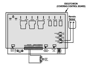
Figure 23 - Remote Temperature Sensor Wiring
