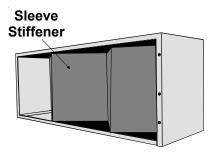
Figure 3 - Wall Sleeve with Stiffener
