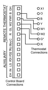
Figure 21 - Wiring Schematic for Remote Heat Pump
