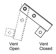
Figure 16 - Vent Door Lever Positions
