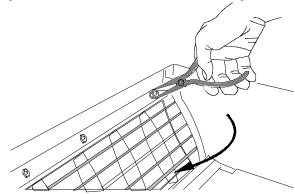
Figure 19 - Discharge Air Flow Grille Removal
