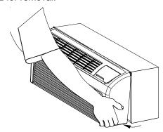
Figure 8 - Cabinet Front Removal View 2
