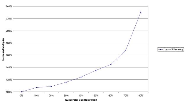
Energy Cost Multiplier Caused by Dirty Filter or Evaporator Coil
