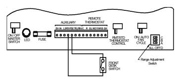
Figure 13 - Front Desk Switch Wiring Schematic
