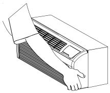
Figure 7 - Cabinet Front Removal View 1
