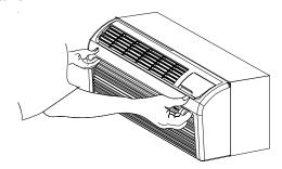
Figure 24 - Opening Intake Grille
