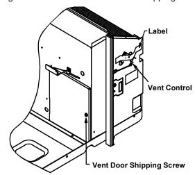
Figure 15 - Vent Control Lever
