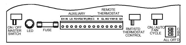
Figure 12 - Control Board User Inputs\*
