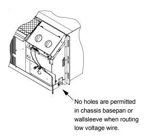
Figure 14 - Low Voltage Wires Routing
