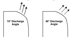
Figure 17 - Discharge Grille Orientation Options
