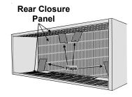
Figure 4 - Stiffener Removal
