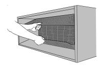
Figure 5 - Rear Enclosure Panel Removal
