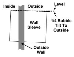
Figure 6 - Proper Sleeve Tilt
