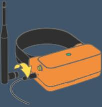
**1** Screw the antenna clockwise onto the threaded connector on Flowie's left side.
